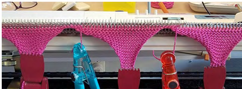
Section 3 complete showing E-wrapped needles
